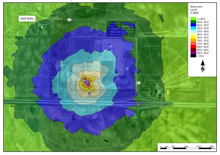
Figure 4. Unmitigated Drilling Noise Contour Map (dBA)
