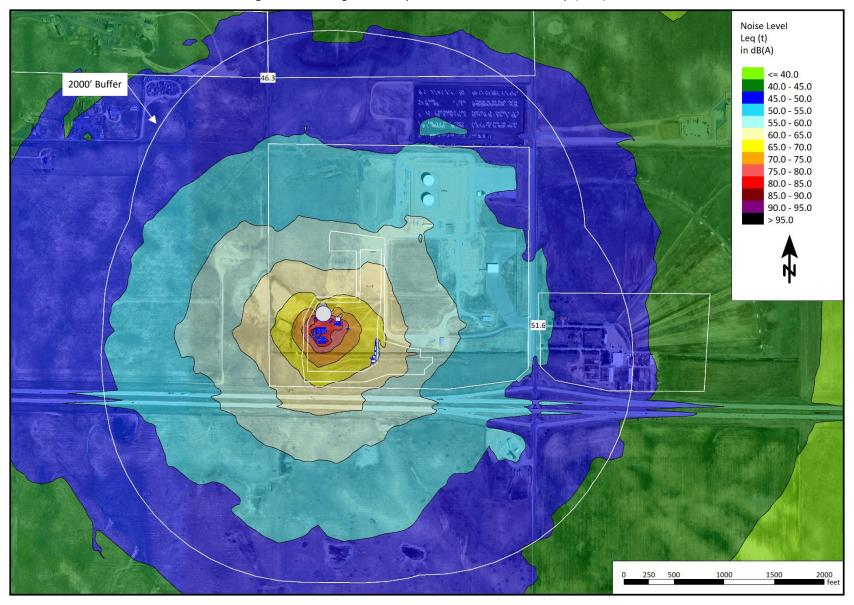
Figure 8. Unmitigated Completions Noise Contour Map (dBA)
