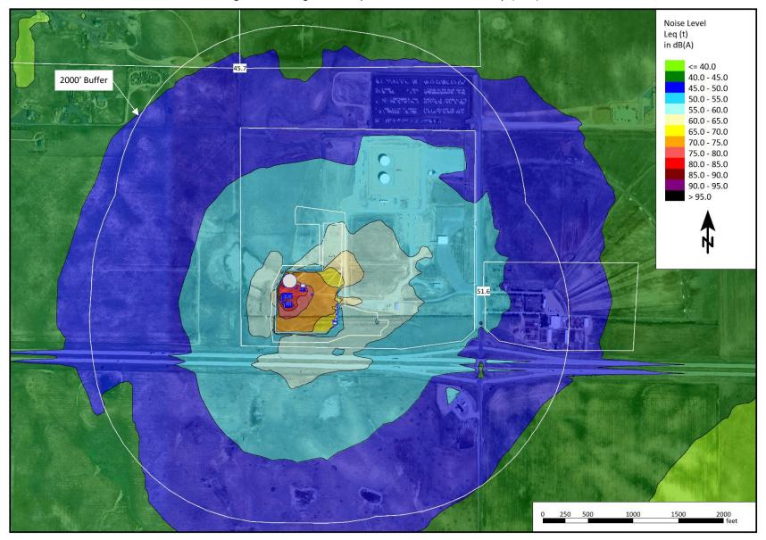
Figure 10. Mitigated Completions Noise Contour Map (dBA)
