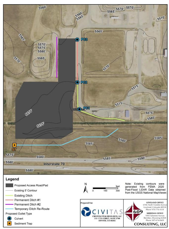
Figure 6. Construction Phase Ditch Locations
