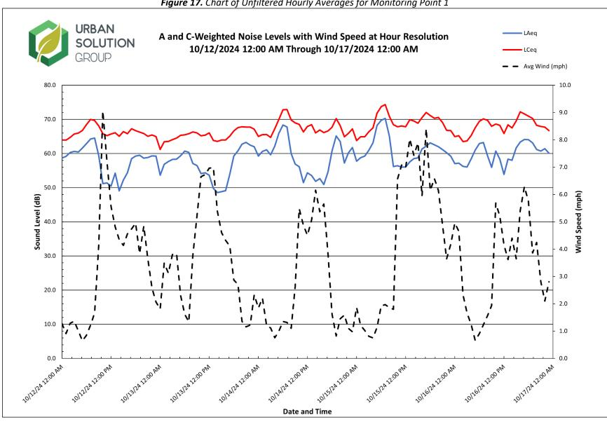
Figure 17. Chart of Unfiltered Hourly Averages for Monitoring Point 1
