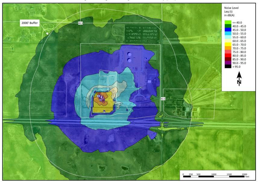
Figure 6. Mitigated Drilling Noise Contour Map (dBA)
