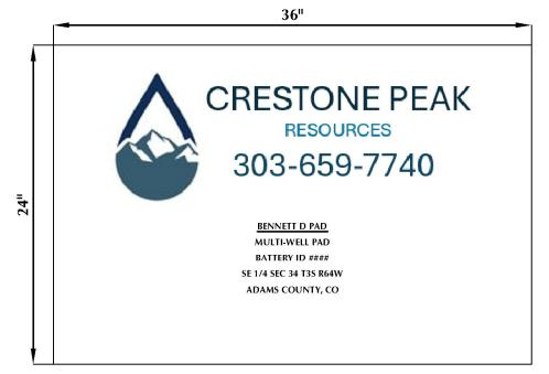
SCALE: NTS SIZE: 36" X 24" MATERIAL: WHITE MAX METAL W/ UV LAMINATE AND CONSTRUCTED ANGLE IRON FRAMES LOCATION: PLACED AT EACH BATTERY
