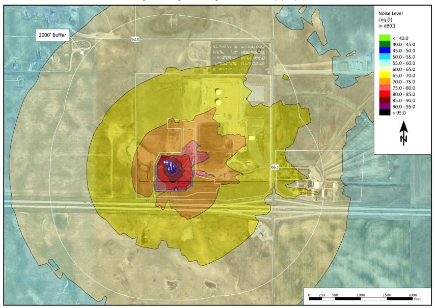
**Figure 7.** Mitigated Drilling Noise Contour Map (dBC)
