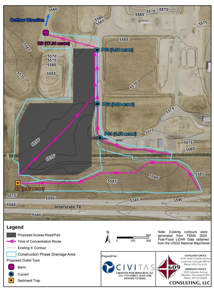
Figure 3. Construction Phase Time of Concentration Routes
