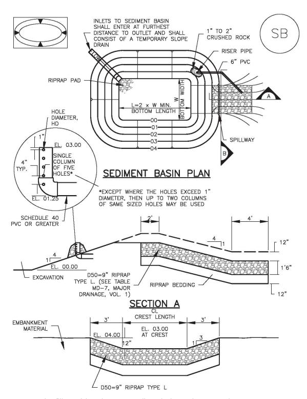
Note: Excavated or fill material used to create a sediment basin must be compacted.
