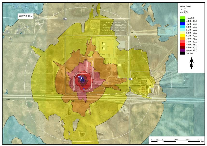
**Figure 5.** Unmitigated Drilling Noise Contour Map (dBC)
