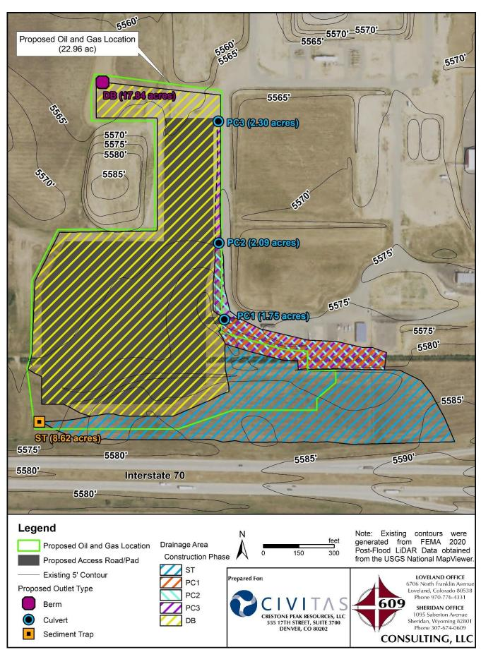
Figure 2. Construction Phase Outlets and Drainage Areas
