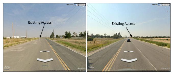
Figure 2. Sight stopping distance. Left picture 400 feet south of the existing access facing north. Right picture 400 feet north of the existing access facing south.
