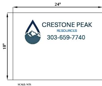
SCALE: NTS SIZE: 24" X 18" MATERIAL: WHITE MAX METAL W/ UV LAMINATE AND CONSTRUCTED ANGLE IRON FRAMES LOCATION: PLACED AT EACH WELL HEAD
