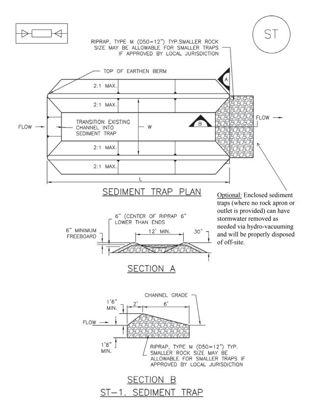
Note: Excavated or fill material used to create a sediment trap must be compacted.
