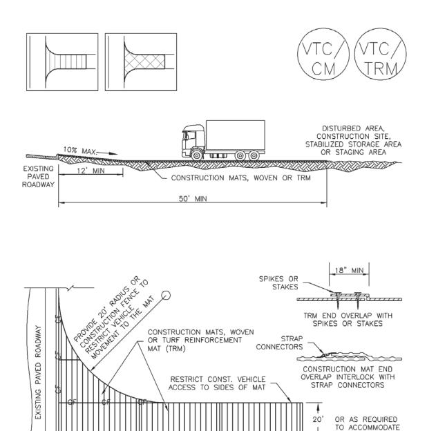
VTC-3. VEHICLE TRACKING CONTROL W/ CONSTRUCTION MAT OR TURF REINFORCEMENT MAT (TRM)
