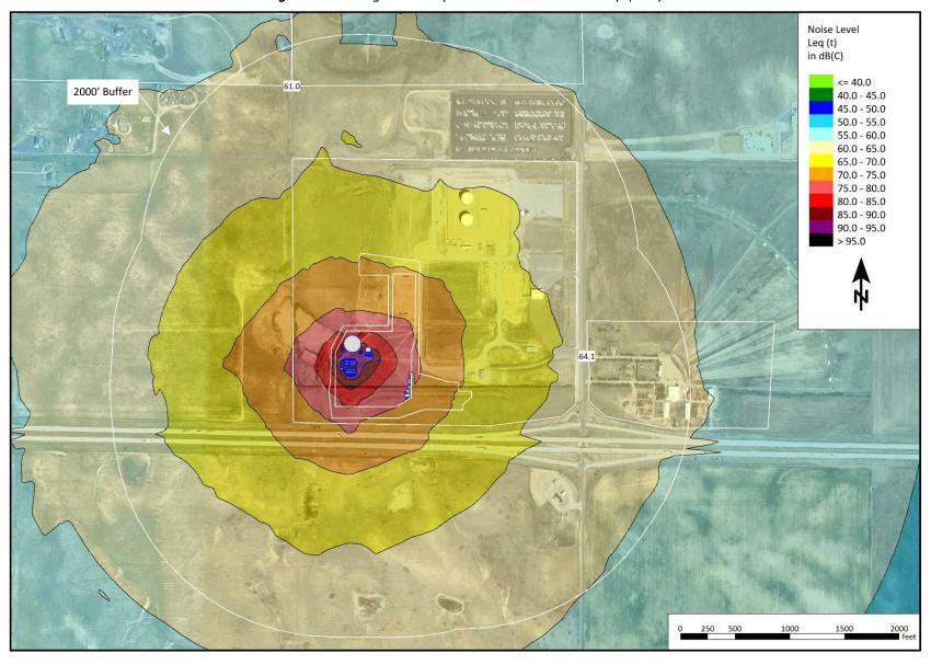
Figure 9. Unmitigated Completions Noise Contour Map (dBC)
